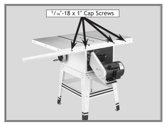
Figure 2. Rear fence rail bracket.
